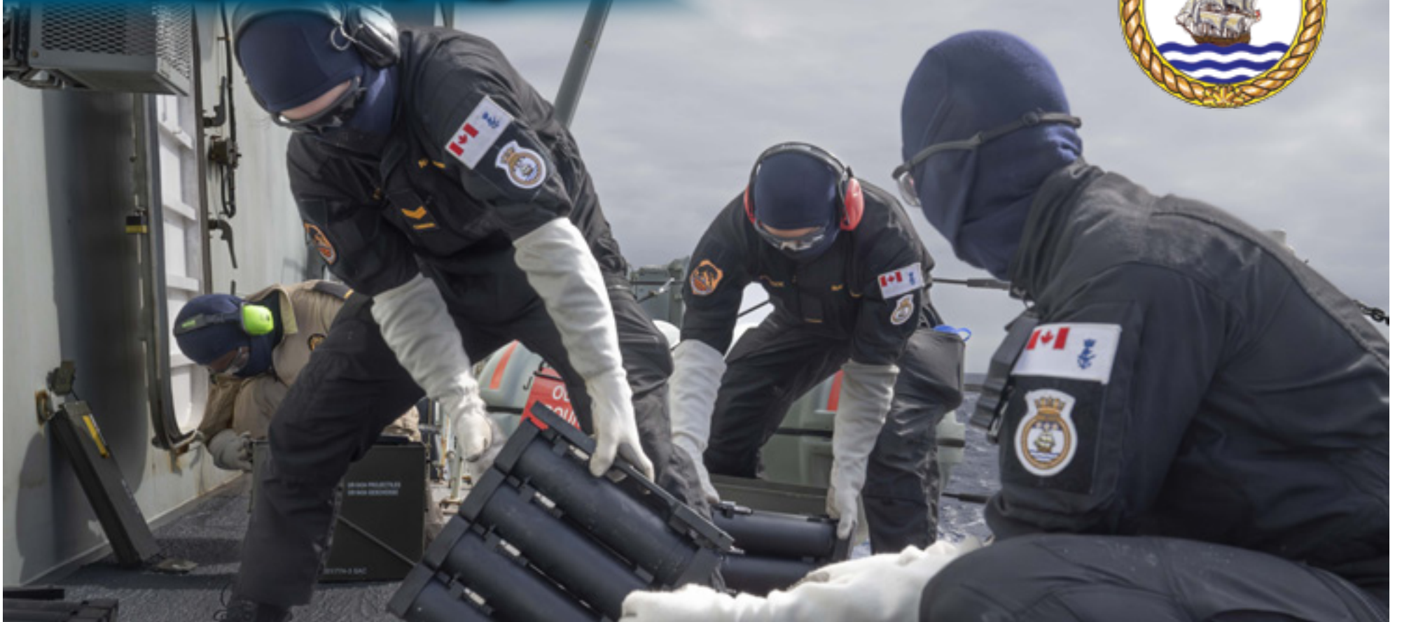
Sailor 1st Class Dean Fisher (Left), Sailor 3rd Class Ryan Stalwick and a Royal Canadian Navy member aboard HMCS Vancouver prepare to reload the multi-ammunition soft-kill system launcher (MASS) during the Technical Cooperation Program Anti-Ship Threat Project Arrangement (TAPA) 2024 while at sea. TAPA is performed every two years, which allows for the testing and training of electronic warfare technology and tactics. Photos: Aviator Conor R.G. Munn, Canadian Armed Forces Imagery Technician.
