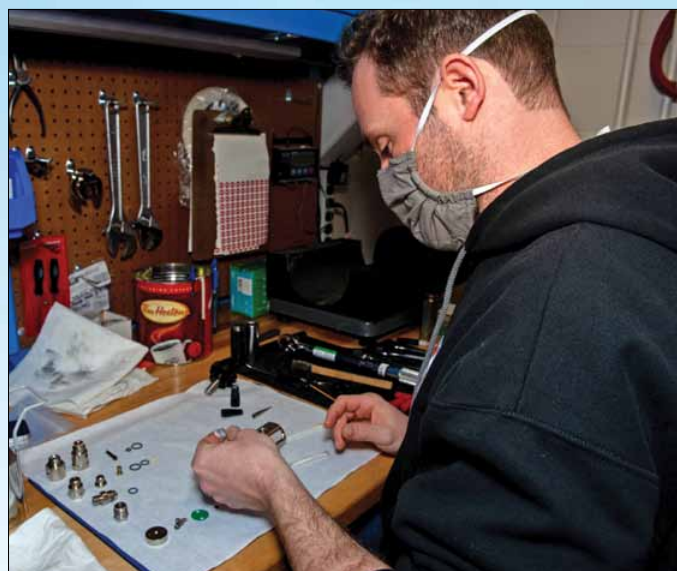
Andy Small rebuilds firing heads for high pressure air bottles.
