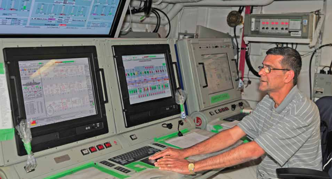
HMCS Calgary was the first of 12 frigates to cycle through the Halifax Class Modernization Frigate Life Extension Program. Noticable highlights on the ship involve significant upgrades to the Machinery Control Room and the Operations Room. Alkarim Nathoo, engineer with L3 Mapps tests the new equipment in the Machinery Control Room. The touch screen monitors will be used throughout the ship.
