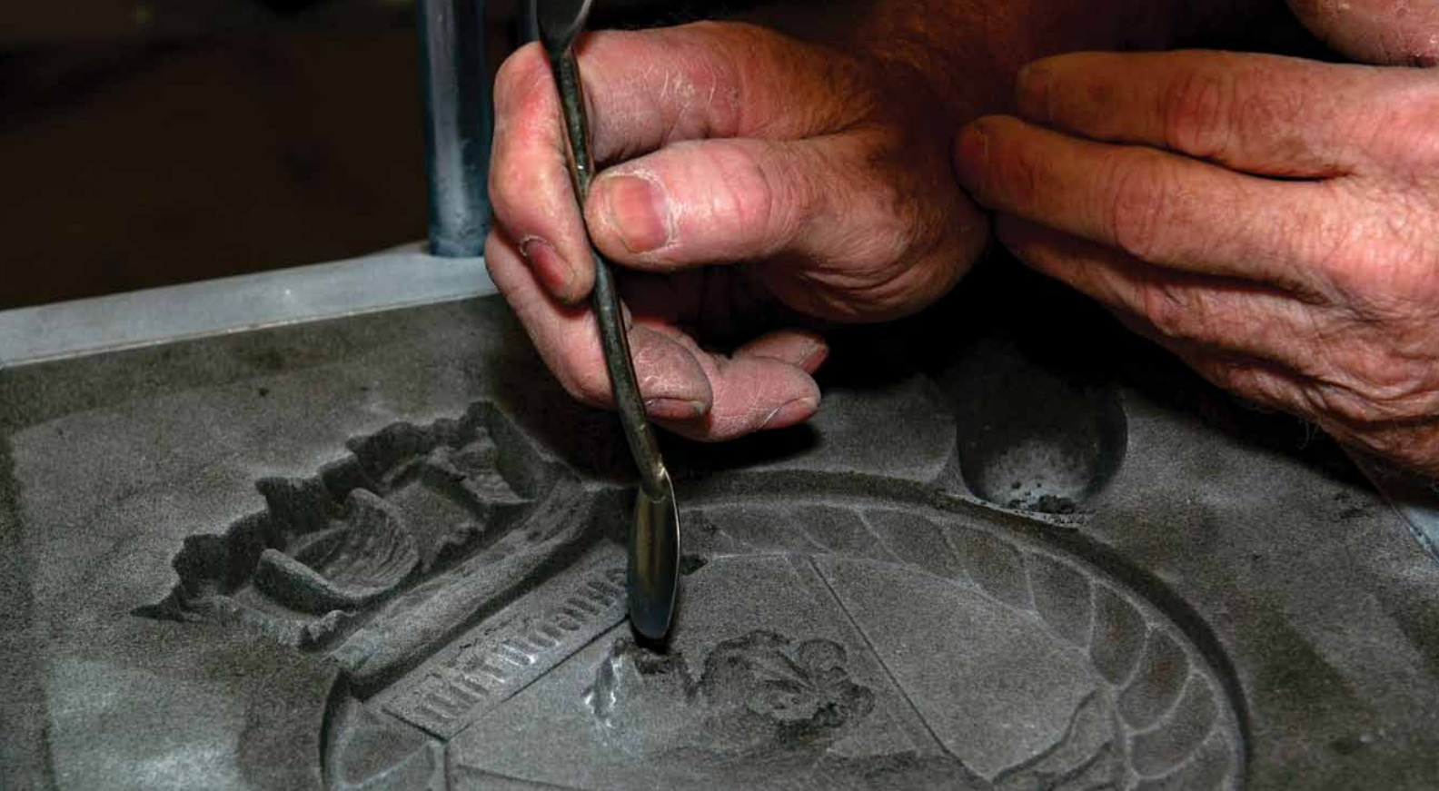
Above: Jack Morgan prepares an aluminum castings in the foundry. Below: A sun dial casting made at the foundry.
